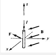
*Example:* a square loop of wire in the z = 0 plane carrying 2 mA in the field of an infinite filament on the *y* axis, as shown. Find the total force on the loop?
