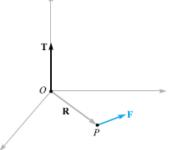
*Example:* A conductor located at x = 0.4m, y = 0 and 0 < z < 2.0 m carries a current of 5.0 A in the  $a_z$  direction. Along the length of the conductor  $B = 2.5a_x$  T. Find the torque about the z axis?
